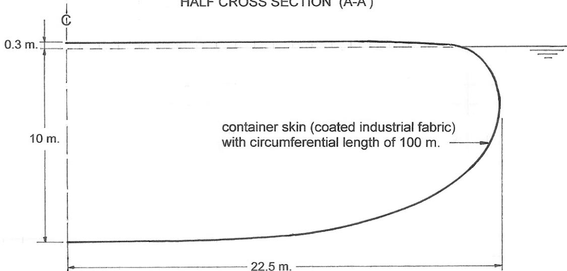
By applying a special method (\*) of compacting the emptied containers, the towage vessel's return voyage to the 'upstream' single point mooring can be undertaken at high speed, close to the vessel's hull speed limit. This minimizes return trip time and maximizes the total volume of water that can be conveyed per towage assembly per year. (\*) patents pending
